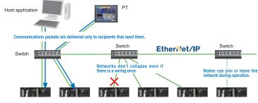
Star topology using Ethernet switch technology
