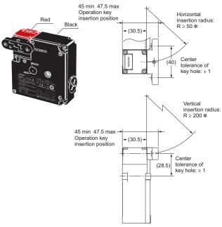
D4NL + D4DS-K3 (with Top-inserted Operation Key)
