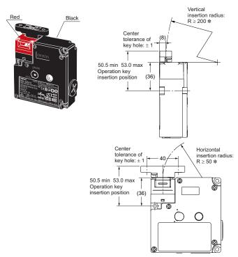
D4NL + D4DS-K5 (with Front-inserted Operation Key)
