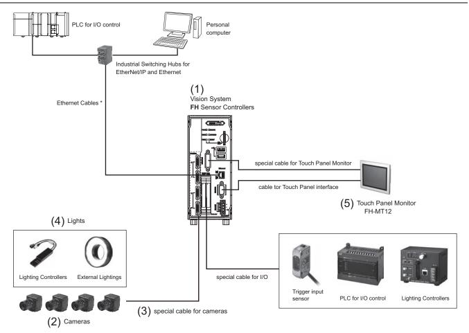
$<sup>^{\</sup>star}$  To use STP (shielded twisted-pair) cable of category 5 or higher for Ethernet and RJ45 connector.
