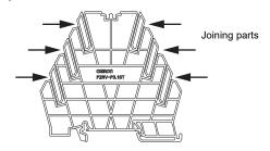
• When removing the PLC interface, place a finger at the place below and pull it out.
