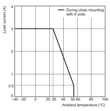
\*When eight or more are installed, install with 10 mm space between each. For details, please refer to *Mounting* on page 27.
