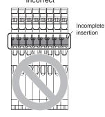
Incorrect installation Some terminals not inserted completely.
