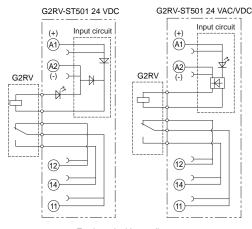
Equipped with a coil surge absorption circuit as standard.
