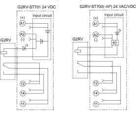
Equipped with a coil surge absorption circuit as standard.
