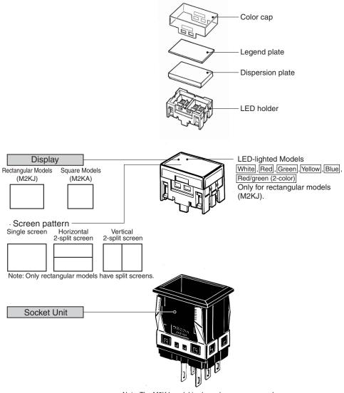
Note: The M2KJ model is shown here as an example.
