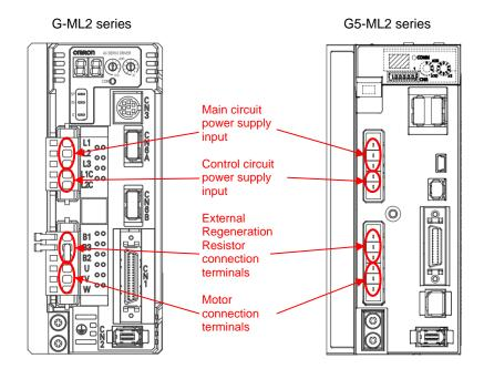
In both the G-ML2 and the G5-ML2 series, input single-phase 100 V and 200 V to the L1 terminal and the L3 terminal.
