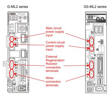
In both the G-ML2 and the G5-ML2 series, input single-phase 100 V and 200 V to the L1 terminal and the L3 terminal.
