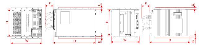
■ Main circuit power supply voltage 200 V drive dimensions
