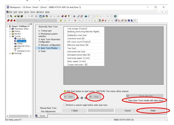
\* If you perform auto tuning with rapid acceleration/deceleration applied to operation commands, Error counter overflow (Alarm No. 24) may be detected.
