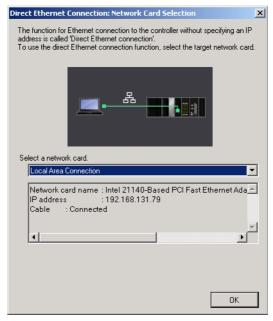
The network card for a direct Ethernet connection is selected and installation continues.
