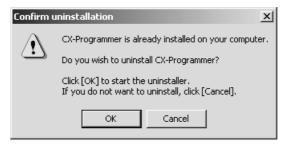
Click the **OK** Button and uninstall the earlier version of the CX-Programmer. If the **Cancel** Button is clicked, CX-One installation will continue without uninstalling the earlier version of the CX-Programmer. This would result in there being two versions of the CX-Programmer installed at the same time, so we recommend always clicking the **OK** Button.
